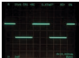
Input: 10 kHz square wave 400 mAp-p (Oscilloscope bandwidth 20 MHz)
