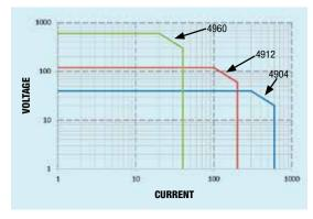
Figure 2 - Discharge Operating Envelope
