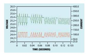
Figure 4 - High Speed Waveform Set (Red) & Capture (Green)
