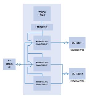
Figure 1 - Independent testing of 2 different battery types
