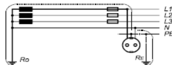
Fig. 56. Presentation of Fault loop in TT- system
